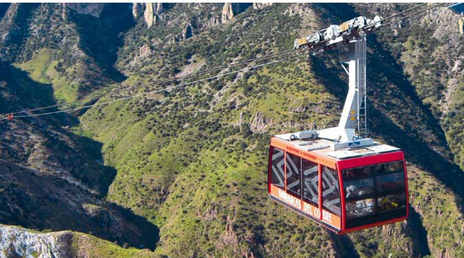
Ropeways, including aerial trams, rank amongst the safest means of transport in existence. This is due to extensive experience and the many safety devices used. Hydrostatic auxiliary or emergency drives ensure that the carriers can be safely brought back to the stations in the event of a failure, such as a power outage. If the tram is blocked, the passengers have to be evacuated from the cabins. This can be done using rope-down devices incorporated in the cabins.
