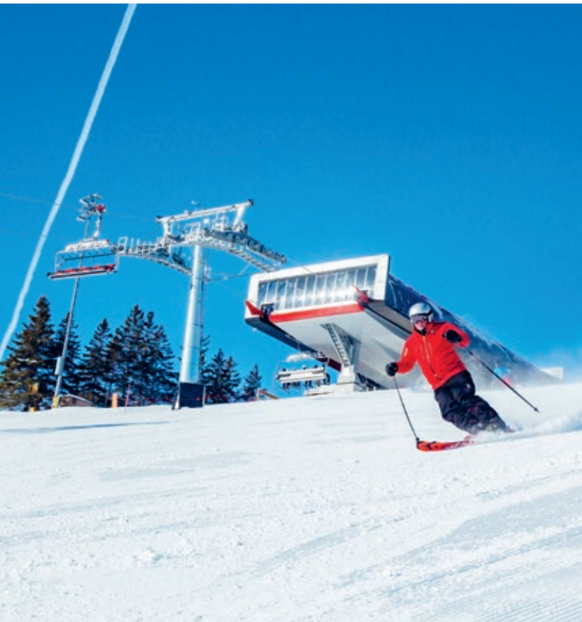
The D-Line 8-seater Adventure 8 shortens previous waiting times with an impressive capacity of up to 4,250 passengers an hour.
