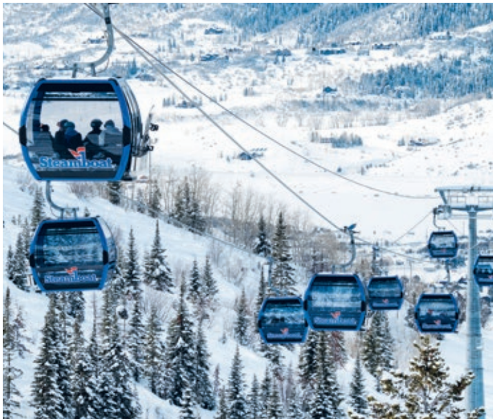
With a total length of over five kilometers, the Wild Blue Gondola is the longest 10-passenger gondola lift in North America.
