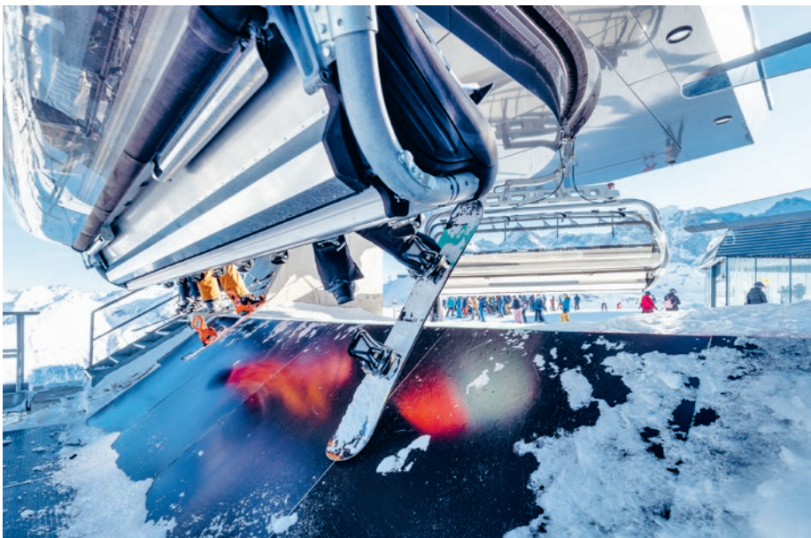
Slide ramps and pressure mats provide additional safety on AURO chairlifts.
