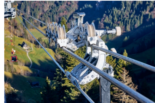
At the heart of the TRI-Line is its newly developed carriage. Two D5000 grips attach to the rope from above while eight carriage wheels – four on each track rope – ensure exceptionally smooth motion and stability.
